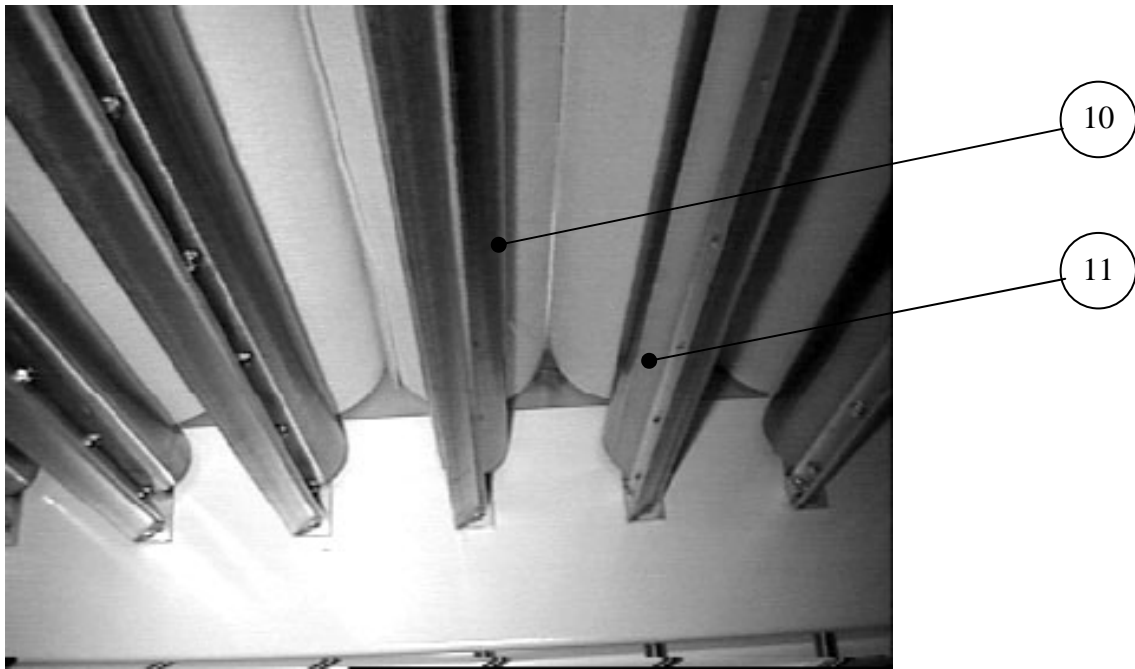
Fig. 4 Squeeze roller with scraper (seen from below)
